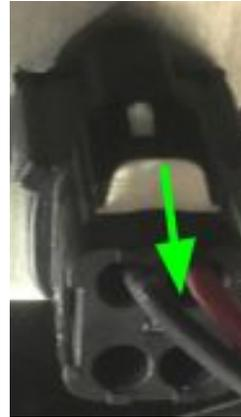
1) Pull the white tab out. It should move ~ 1/4th inch. But it will not completely separate from the connector.
