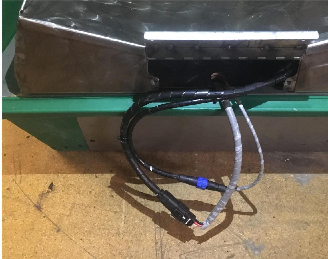
Unscrew the blue nuts from one another to disconnect the first cable
