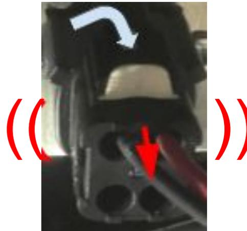
2) Push down on the black tab and wiggle the connector while pulling it apart.
